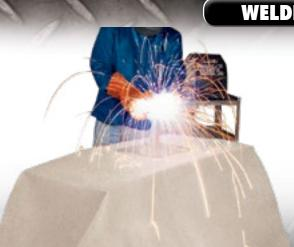
Welding blankets and rolls are widely used for draping over equipment or floor surfaces in welding areas, or as a vertical shield to protect from sparks, spatter, and slag.
