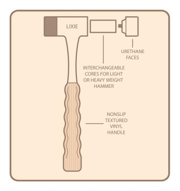
**Configurations:** Lixie Unihammer's are available in two (2) weights and numerous face hardnesses to meet your specific application requirements.
