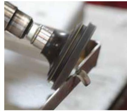
Edge chamfering a fabricated stainless component.
