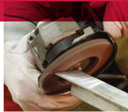
Chamfering an aluminum extrusion preparing for weld
