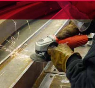
Smoothing the edges of rollercoaster track with a resin fiber disc.
