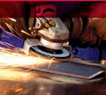
Grinding & blending a weld between two Steel plates.
