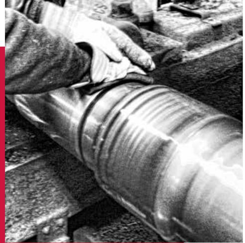
All non-woven products are fabricated from base materials that are composed of a random "web" of nylon fibers that have been bonded together with synthetic resins and impregnated with abrasive grains. Although these materials vary in fiber density, their three dimensional nature results in specialty abrasive products that are pliable, conformable to the work surface, and limited in their ability to remove base stock.
