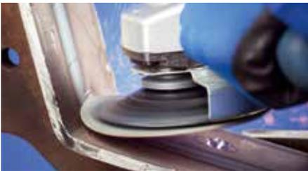
Soft and particularly flexible grinding performance in face-down grinding.
