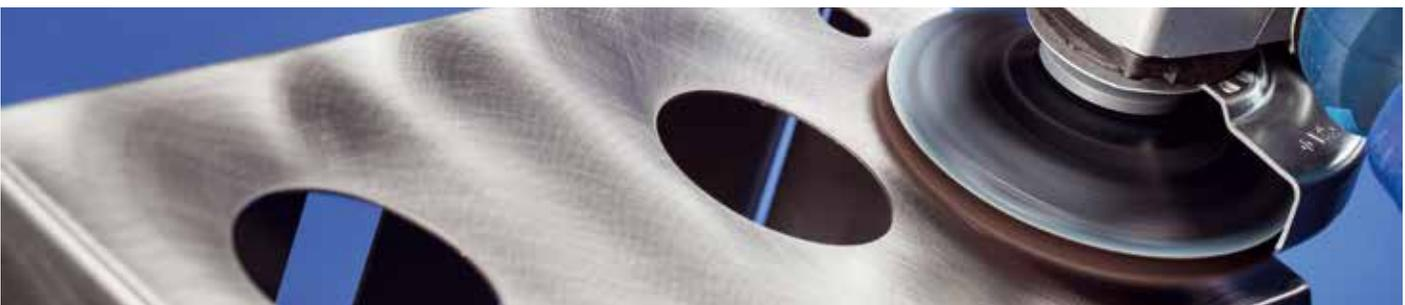
For pre-polishing and high-gloss polishing of medium- to large-sized components, PFERD provides COMBICLICK® felt discs in a range of diameters.
