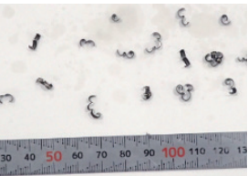
Remaining pip in the center : \phi .056 inch RZ : .0006 inch
