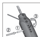
Fig.5 How to use adjustment pin
