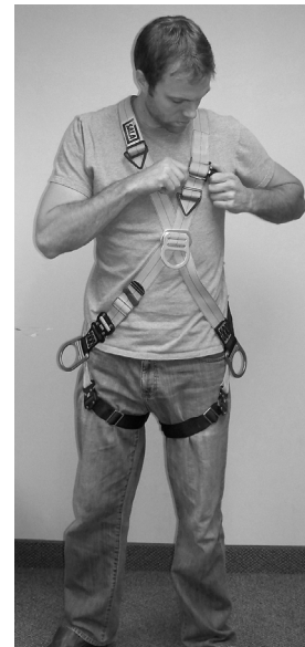
Figure 12 - Installing the Belt (Crossover-Style)
